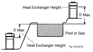
**NOTE:** If heater is installed outside of the limits shown, a flow switch must be used in place of the pressure switch when mounted and wired adjacent to the heater.
